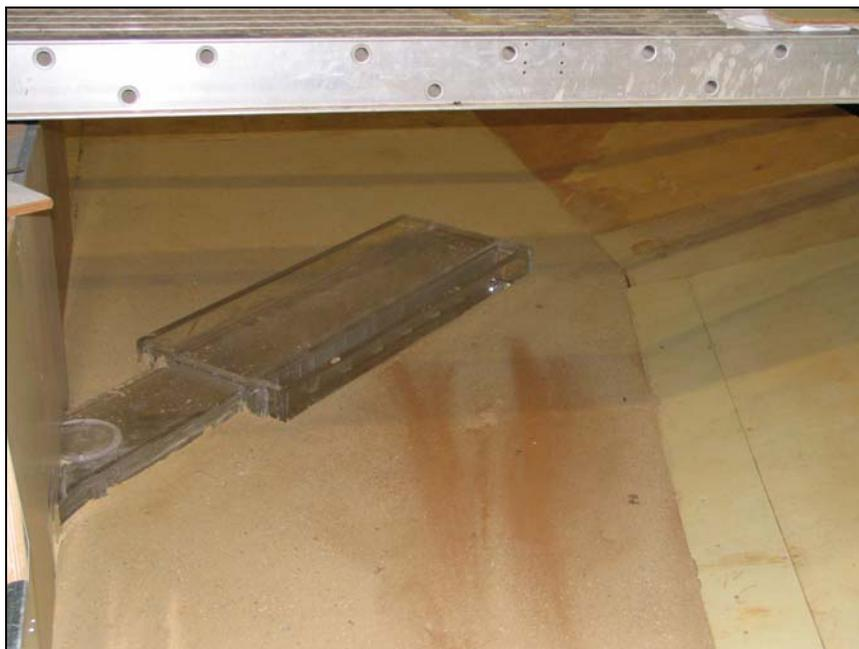
Figure 15. Looking downstream at sand placed around type 13 outlet design.
