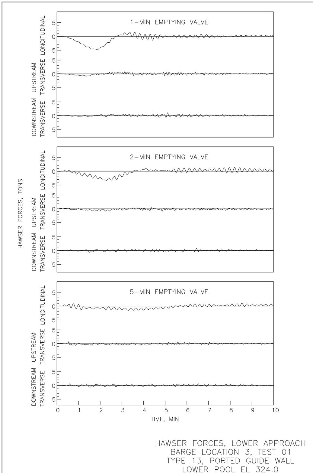
Figure 27. Time histories of hawser forces with alternative 2 lower guide wall at location 3.
