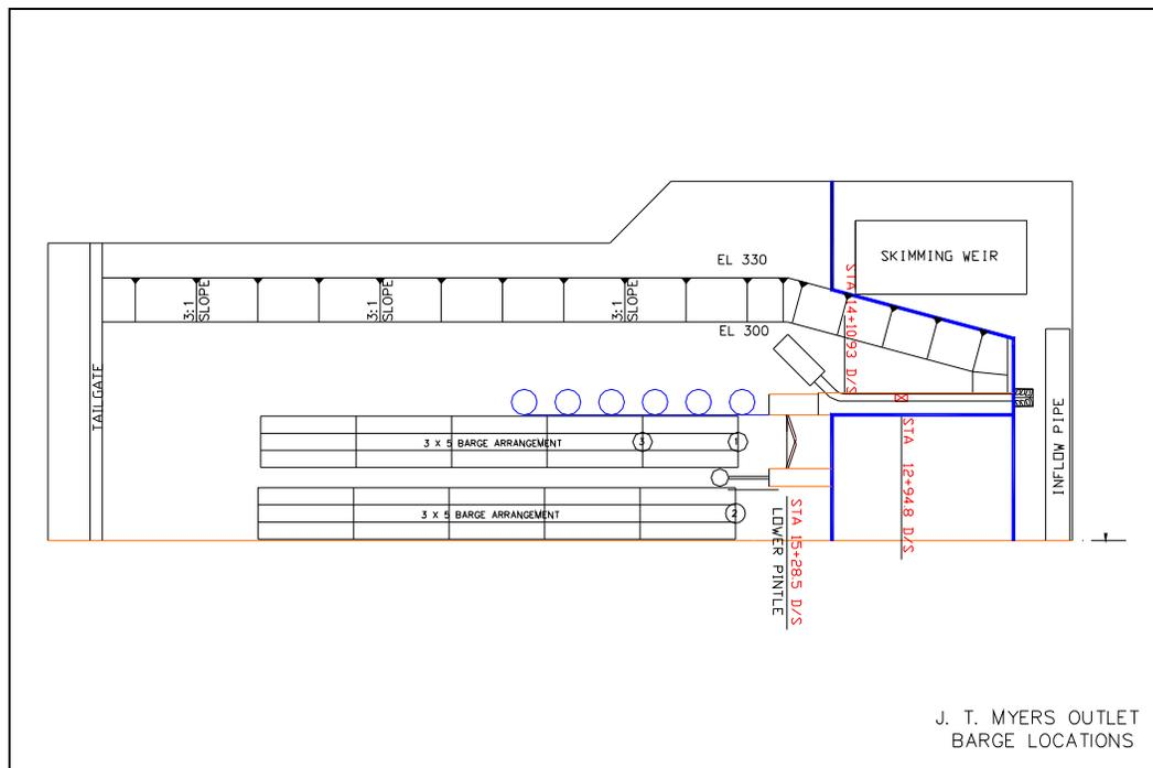
Figure 18. Barge locations for hawser force measurements.
