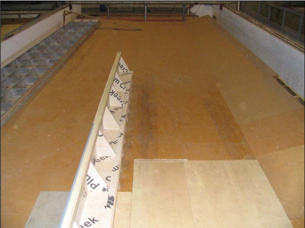
Figure 6. View of 1:25-scale J. T. Myers outlet model looking downstream
