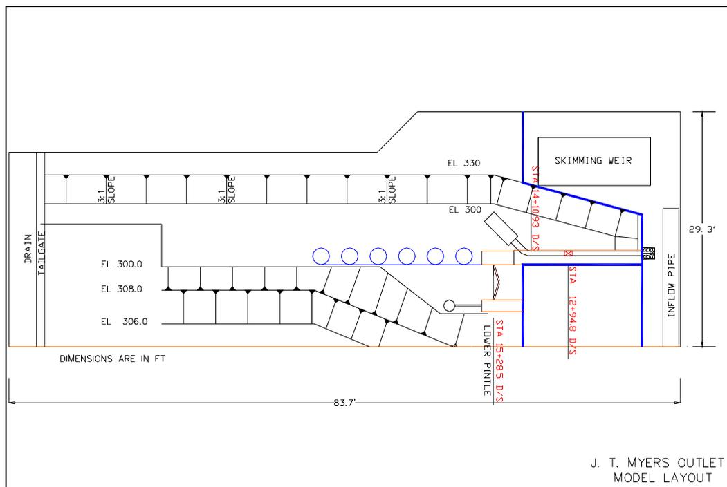
Figure 4. Model layout for landside outlet diffuser
