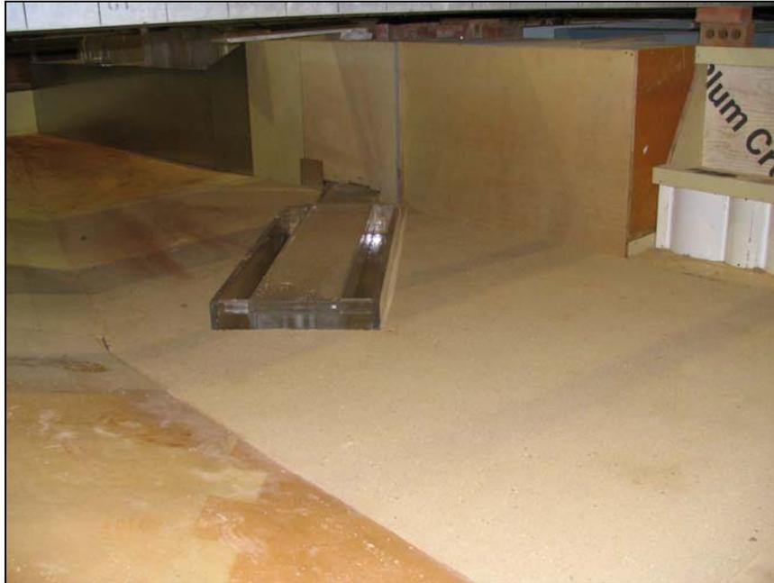
Figure 14. Looking upstream at sand placed around type 13 outlet design.
