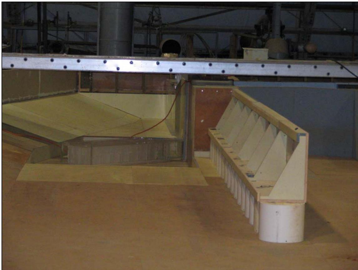
Figure 12. Landside view of Alternative 1 lower guide wall in model looking upstream.
