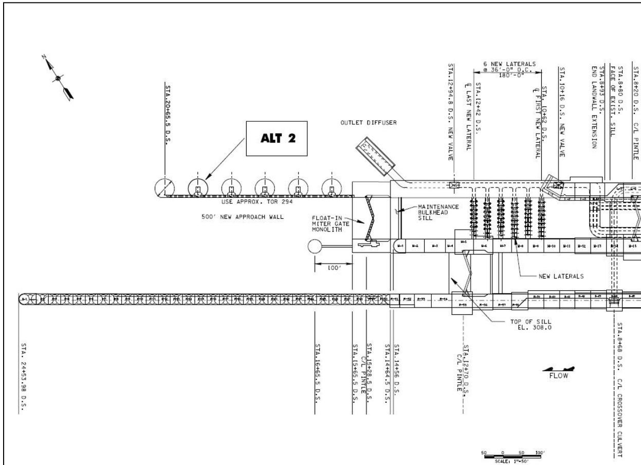
Figure 22. Plan view of alternative 2 lower guide wall.
