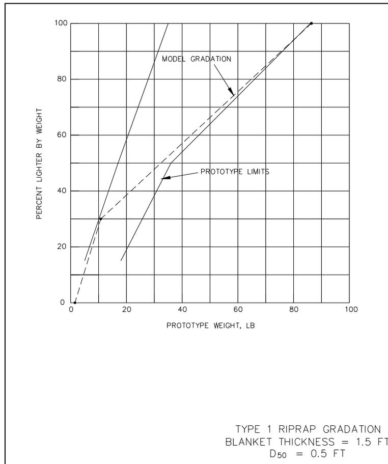
Figure 28. Type 1 riprap design from Hite 2004.
