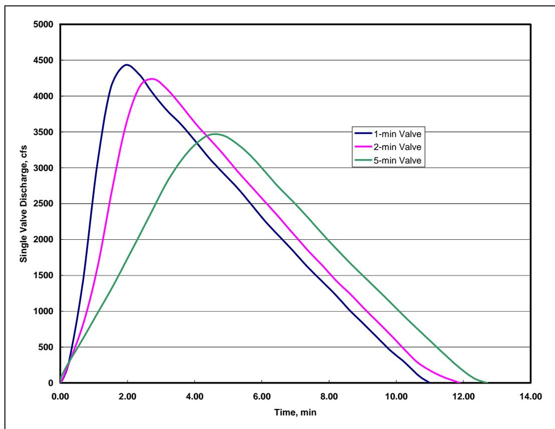
Figure 13. Discharge hydrographs for 1-, 2-, and 5-min valve operations.
