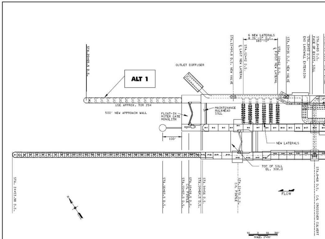
Figure 10. Plan view of Alternative 1 lower guide wall.
