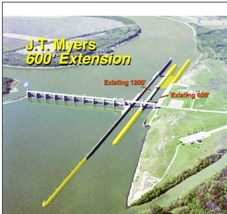
Figure 2. J. T. Myers proposed lock extension looking downstream.
