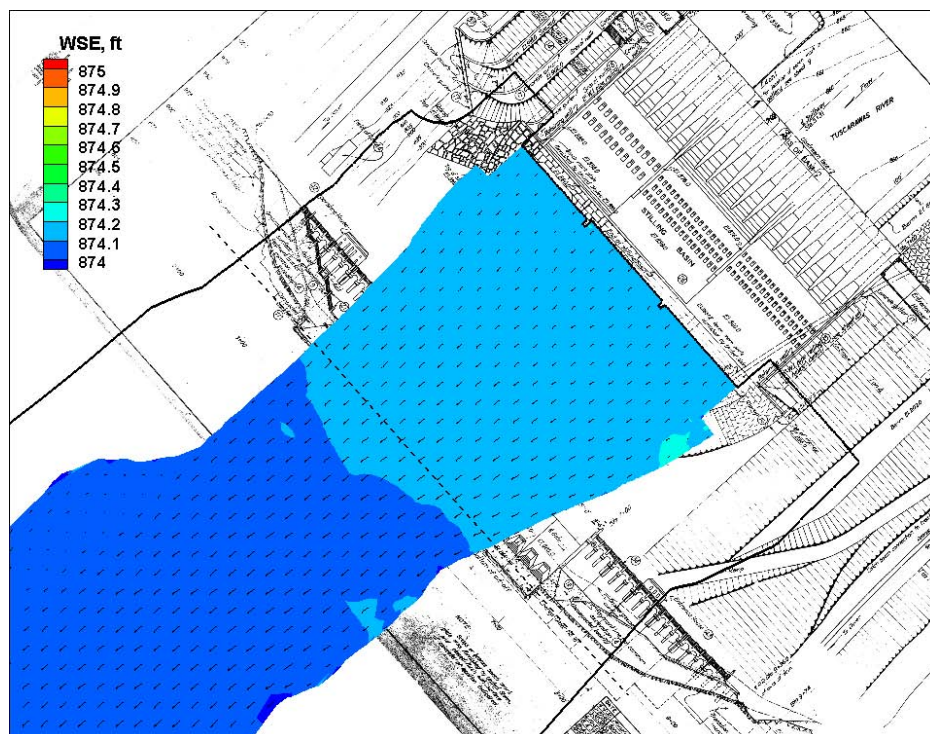
Figure 44. Water surface contours and vectors, flow Condition 7, discharge 8,900 cfs, stilling basin tailwater el 874.1.
