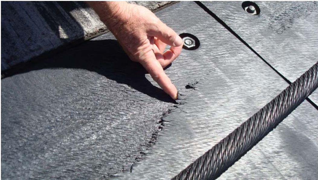
Figure 17. Damage to polyethylene panel likely caused by cable beating on surface of panel at Davis-Monthan AFB.
