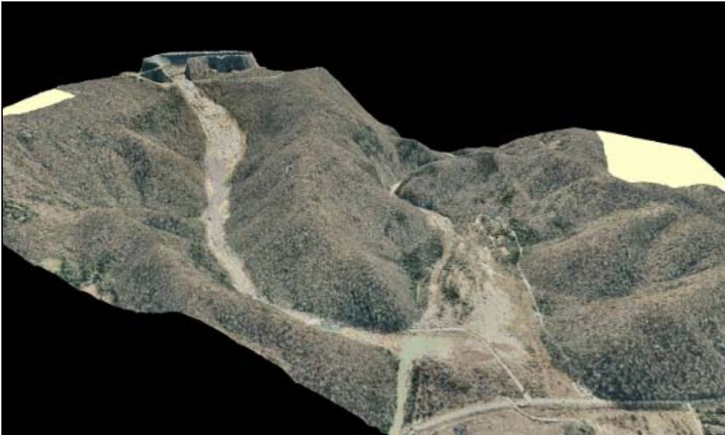
Figure 21. High-resolution imagery overlain on LIDAR-derived surface. The wall failure and stream scour are quite visible even in this overview of the area (Luna et al. 2007).
