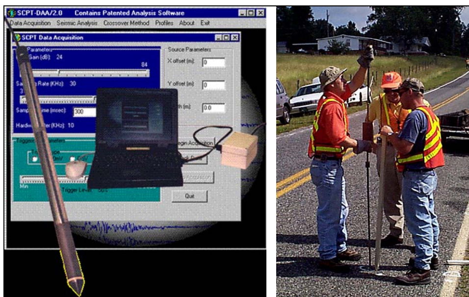
Figure 19. Commercially available cone penetrometer and software system and its use in the field.
