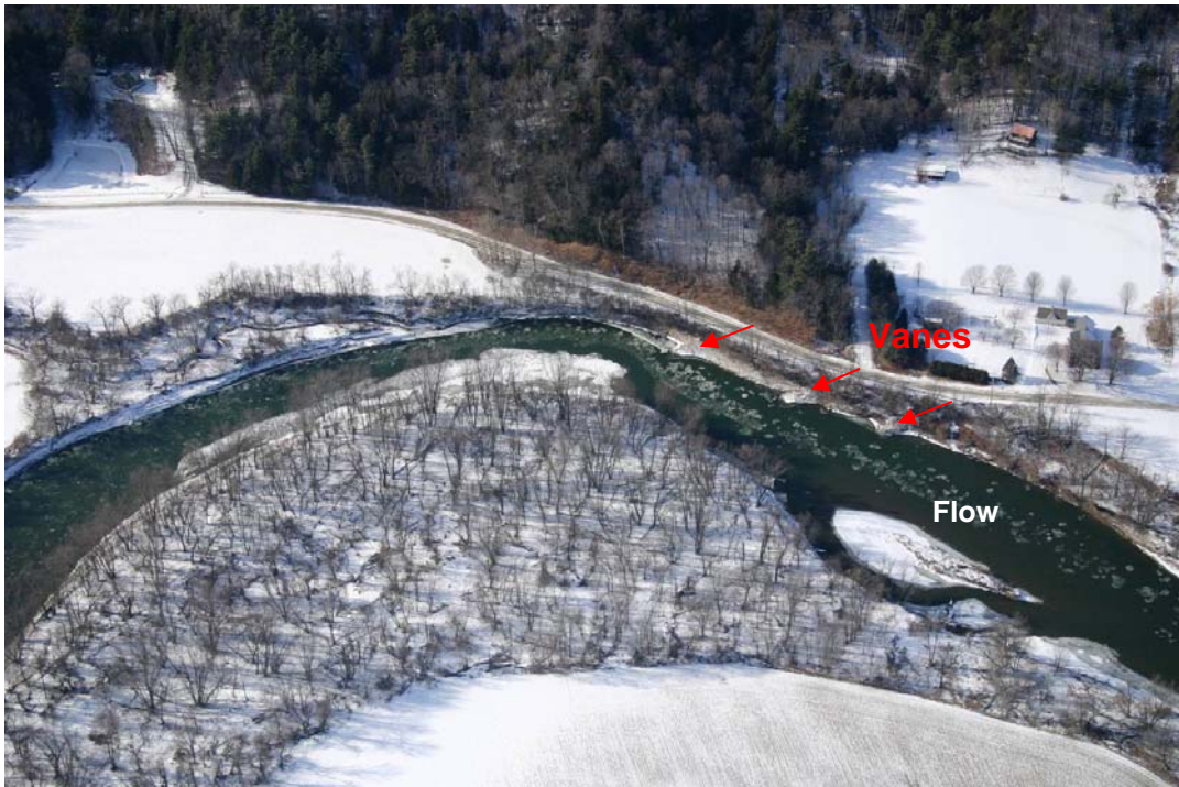
Figure 20. Drifting frazil ice and shore ice forming around vanes and on the Winooski, R. at Gov. Chittenden Rd. vanes, 1/31/08.
