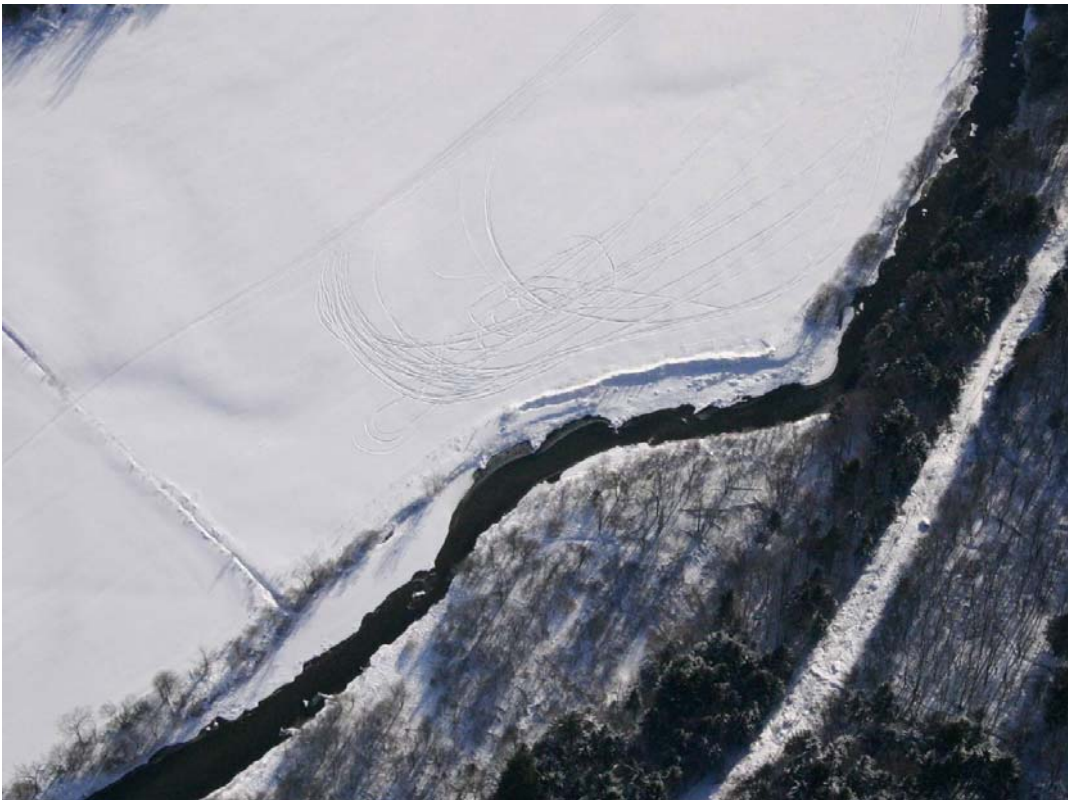
Figure 42. Ice forming around rock vanes in the White River above Rochester, VT, 12/21/05.
