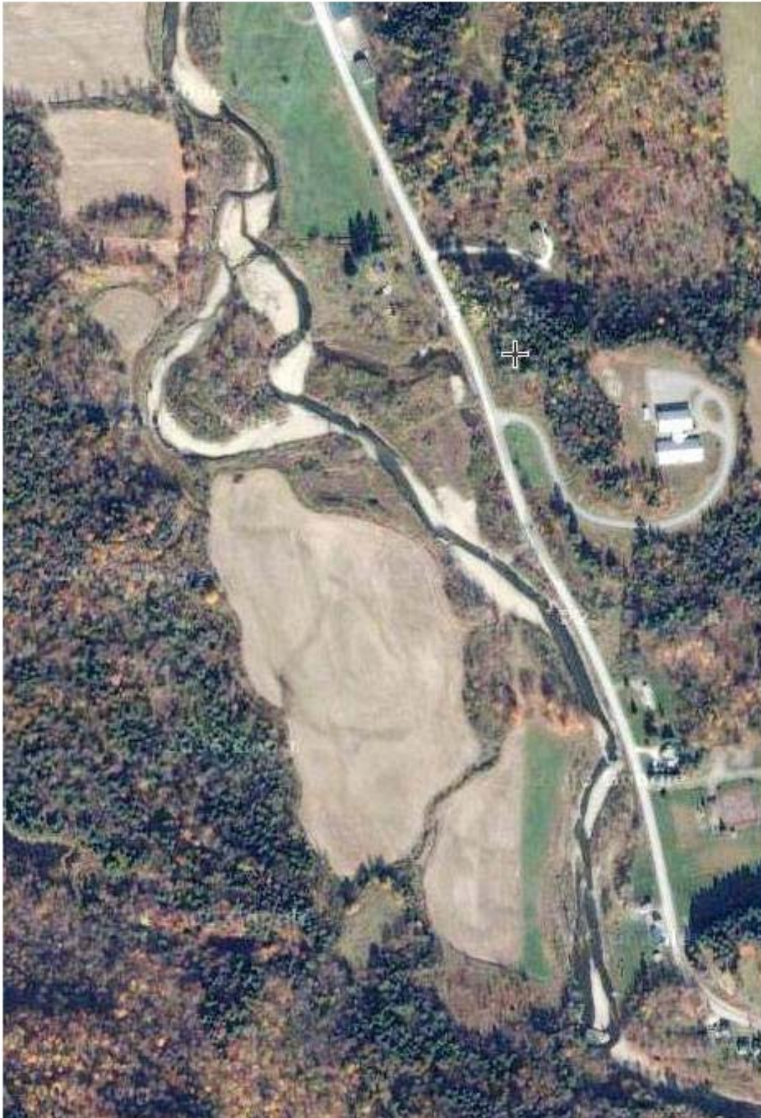
Figure 32. Recent air photo of Trout River restoration project below Montgomery Center. Deposition of coarse material in large meander during October 2005 flood caused a channel avulsion into the former channel area to the right.
