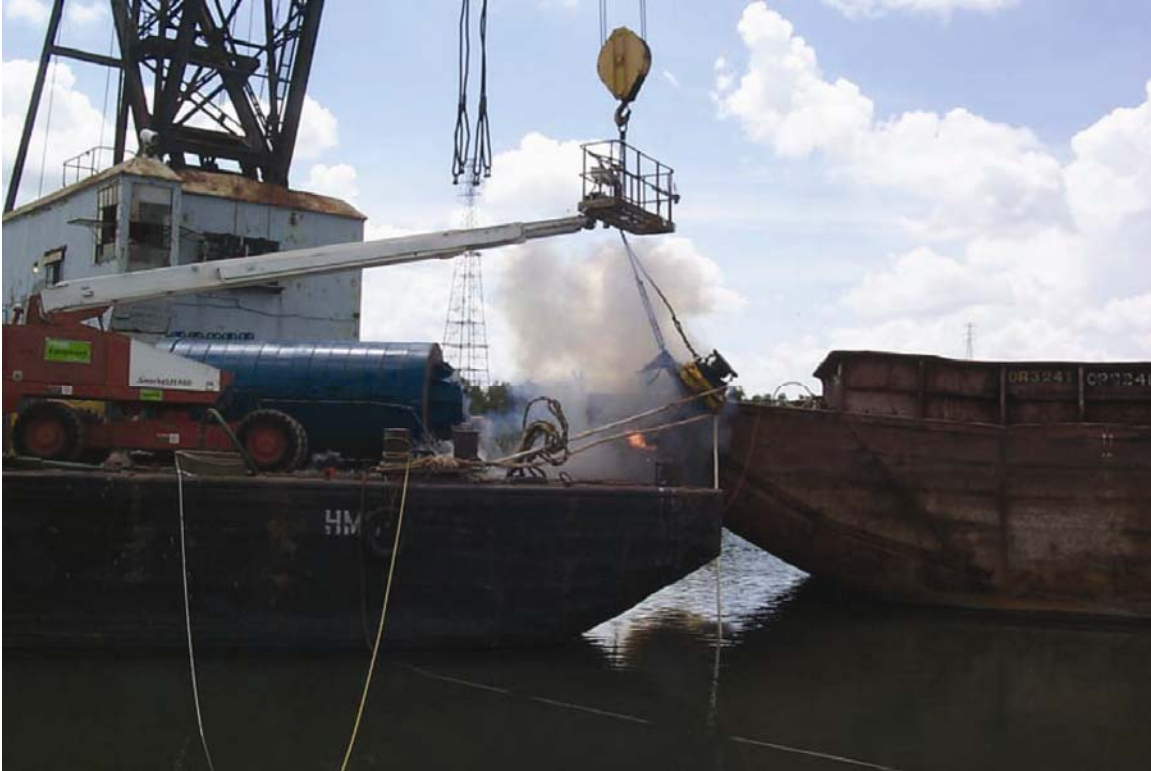
Figure 3.20. Statnamic device and experimental setup during experiment (Note: The detonation of the Statnamic device had just occurred at the time of the photograph) ((HQUSACE 2004)).
