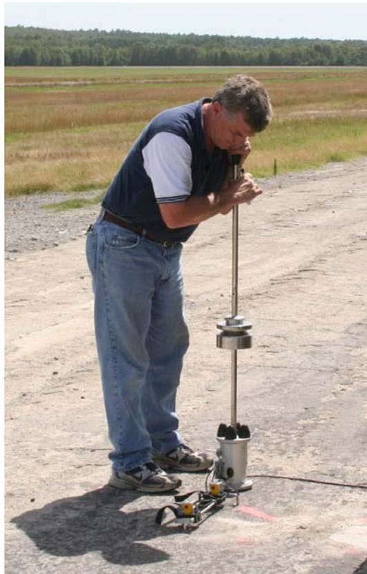
Figure 4. Testing stabilized surface using PFWD.
