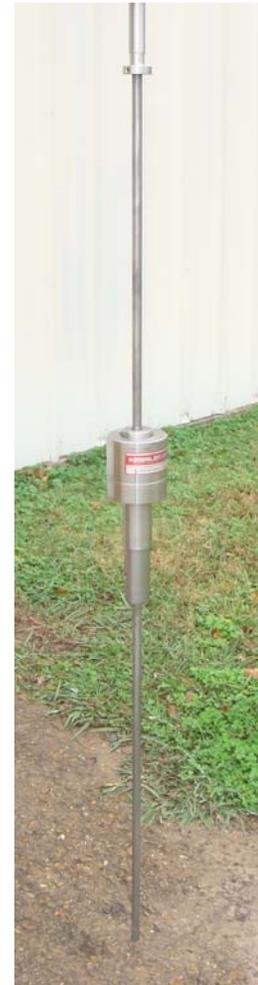
Figure 2. Dynamic cone penetrometer.
