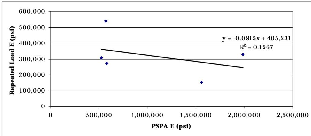
Figure 24. PSPA repeated-load modulus correlation.
