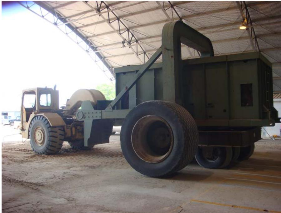
Figure 31. C-17 load cart trafficking stabilized test section.
