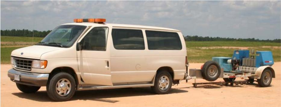
Figure 9. Falling-weight deflectometer testing of stabilized surface.
