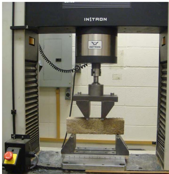
Figure 7. Flexural strength testing using third-point loading.
