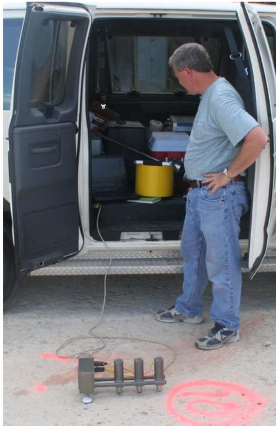
Figure 5. Testing stabilized surface with the PSPA.
