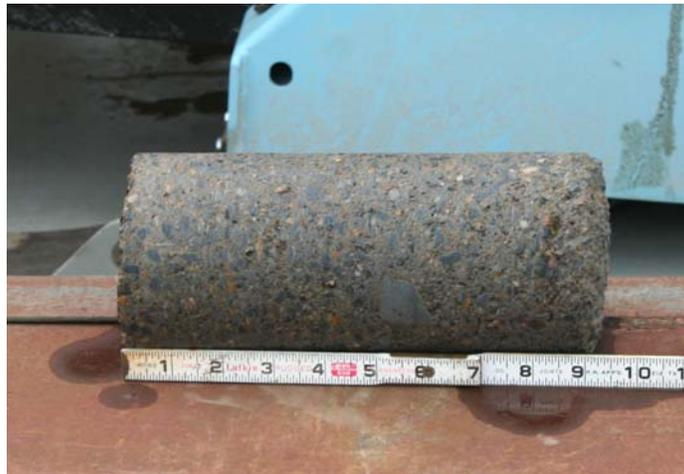
Figure 11. Core sample recovered from existing airfield.
