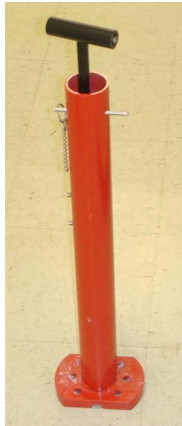
Figure 1. Standard Clegg hammer.
