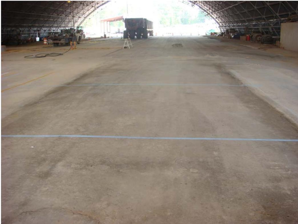
Figure 30. VTS cement-stabilized soil test section.
