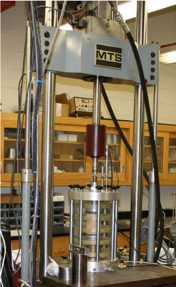
Figure 8. Cyclic triaxial testing on stabilized soil sample.
