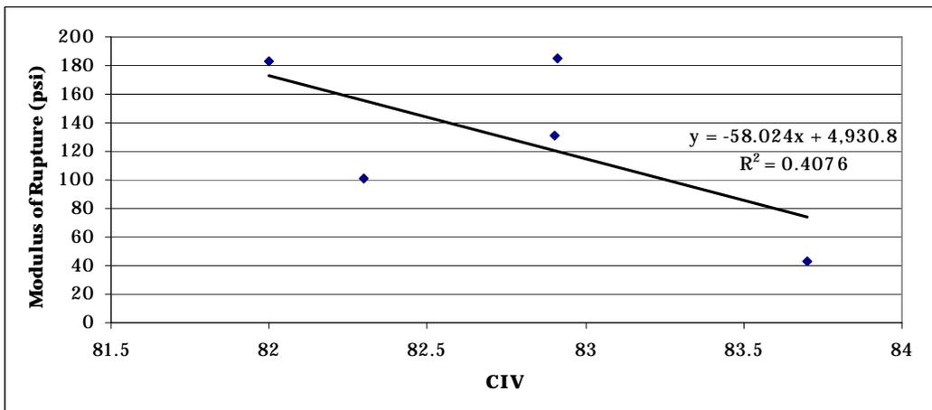
Figure 17. Clegg hammer modulus of rupture correlation.
