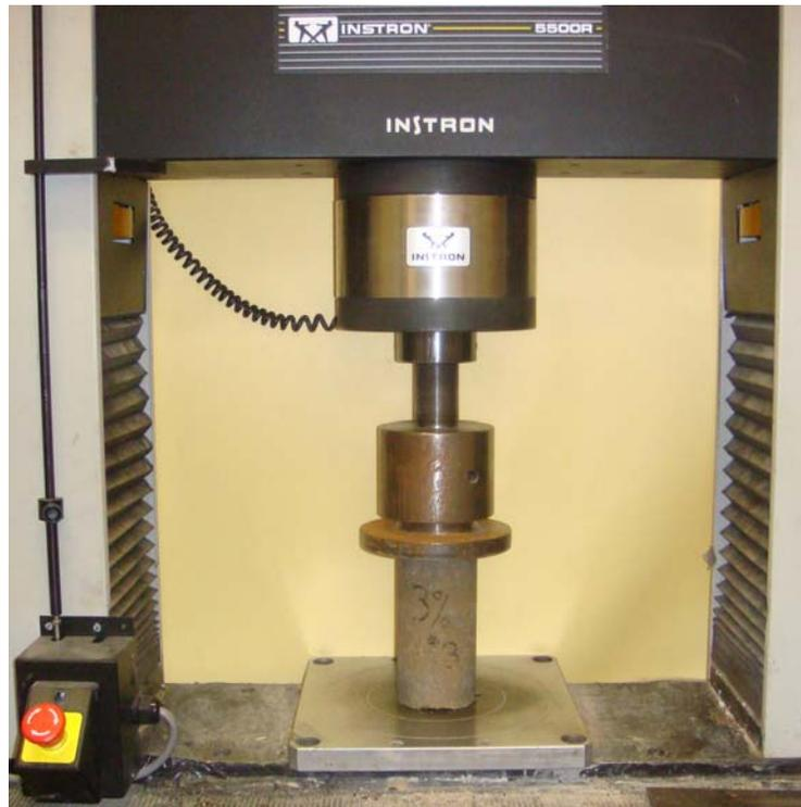
Figure 6. UCS testing on sample.
