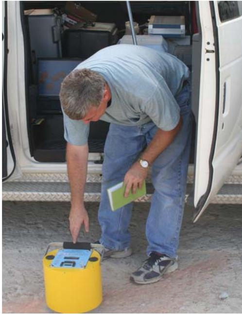
Figure 3. Testing stabilized surface with SSG.
