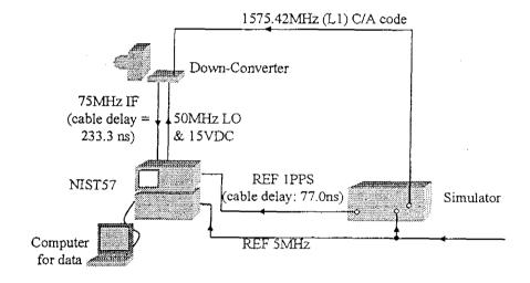
Figure 1. Test setup for the absolute calibration of NIST57.
