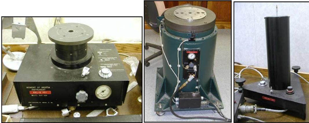
Figure 10. Small-, medium-, and large-caliber MOI measurement devices.
