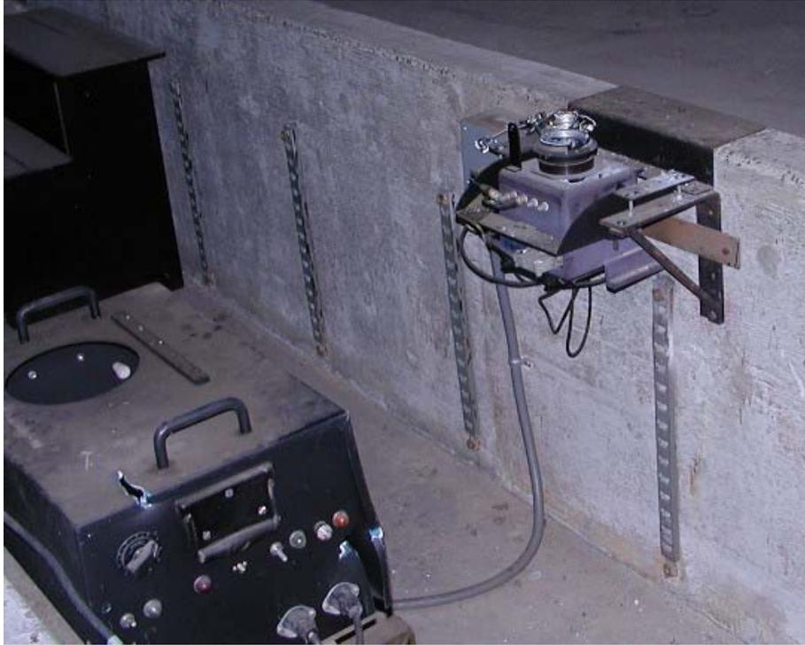
Figure 12. Damaged spark generator and camera in spark range.
