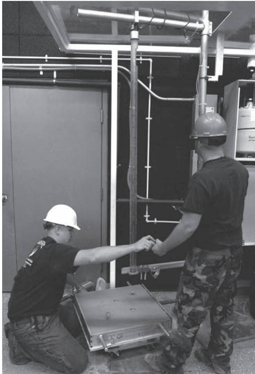
Figure 3: Clay Being Calibrated with Pre-Test Drops
