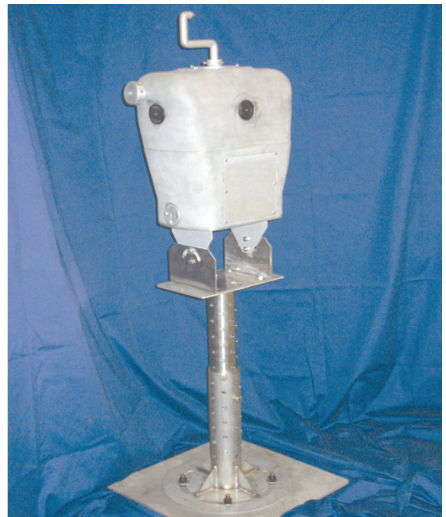
Fig. 10-9. Blast Test Device. Photograph: Courtesy of L-3/Jaycor, San Diego, California.
