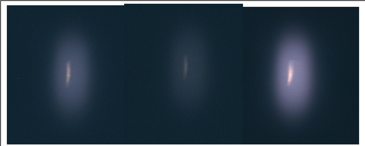
Figure 16. Linewidth Detection of three different 243 nm single shot on to a CCD camera. Please note the halo around the center of the rectangular image is due to fluorescence. The position of each shot did not move as we observed in realtime the shot to shot stability. The size and scale of the image is the same for each shot.
