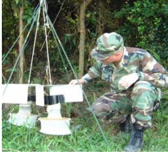
Figure 15. CDC Fay-Prince trap suspended from tripod
