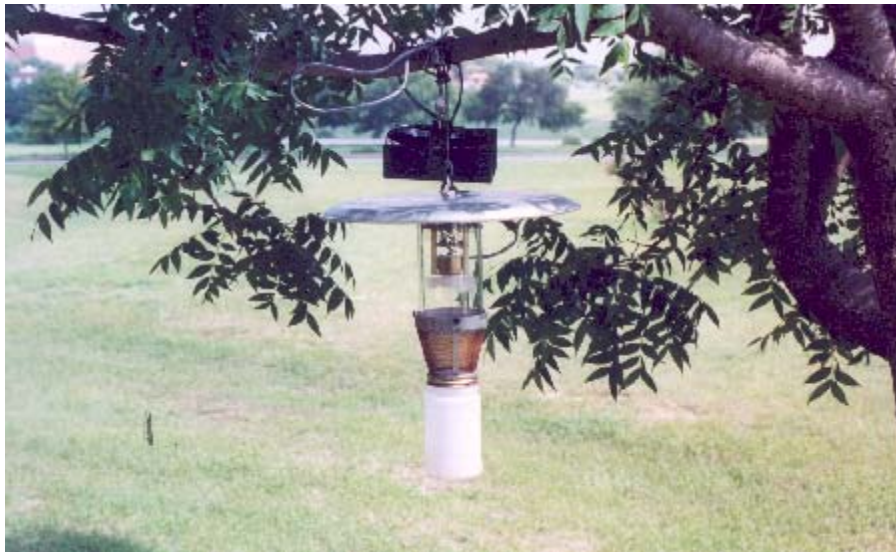
Figure 3. SSAM trap with collection jar shown properly suspended from tree limb
