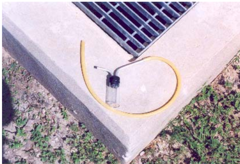
Figure 32. A traditional, mouth-operated aspirator
