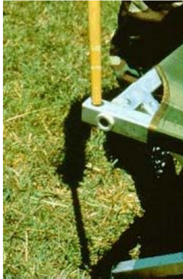
Figure 80. Insert tapered end of support post into corner hole
