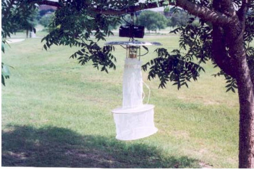
Figure 6. SSAM trap with collection net shown suspended from tree limb
