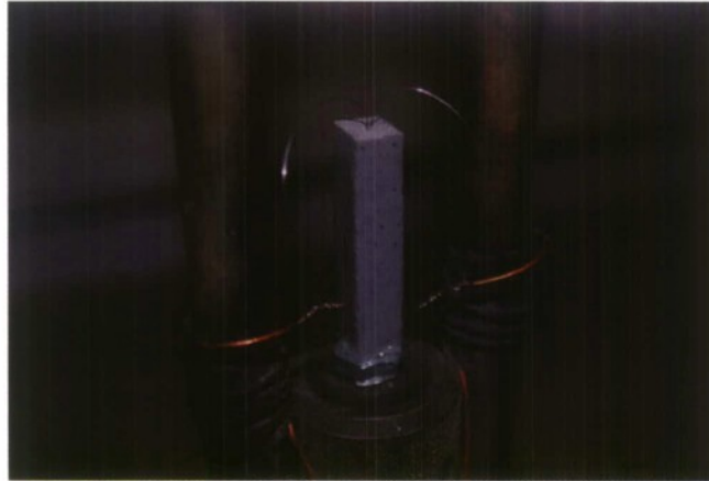
Figure 15: Inhibited propellant prepped to go into Crawford bomb. Shown also is NiChrome ignition wire.
