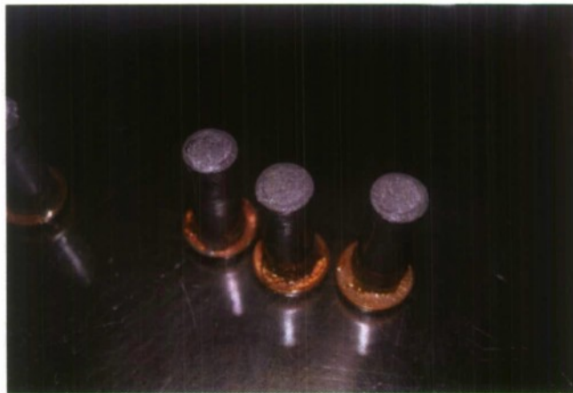
Figure 13: Propellant cast in quartz tubes.
