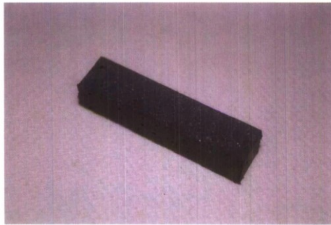
Figure 14: Propellant cut from cast block.
