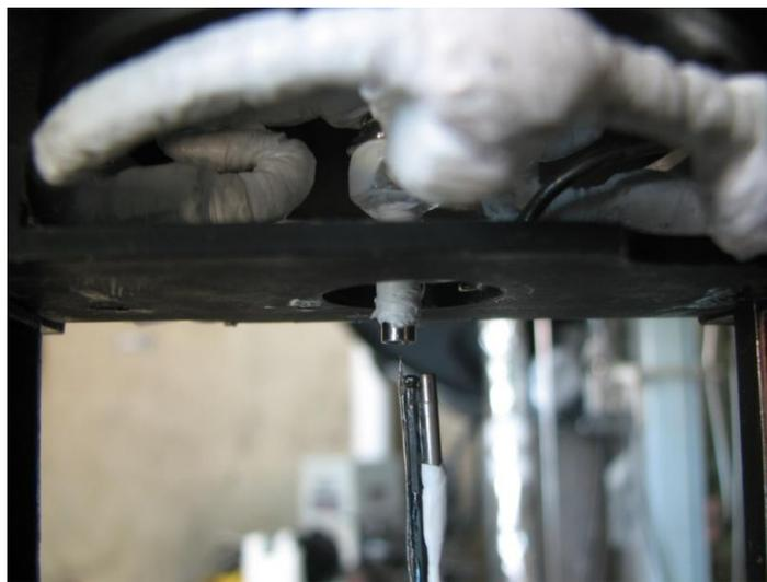
Figure 4.6. Thermocouple and pressure transducer probes near the exit of the coaxial injector.
