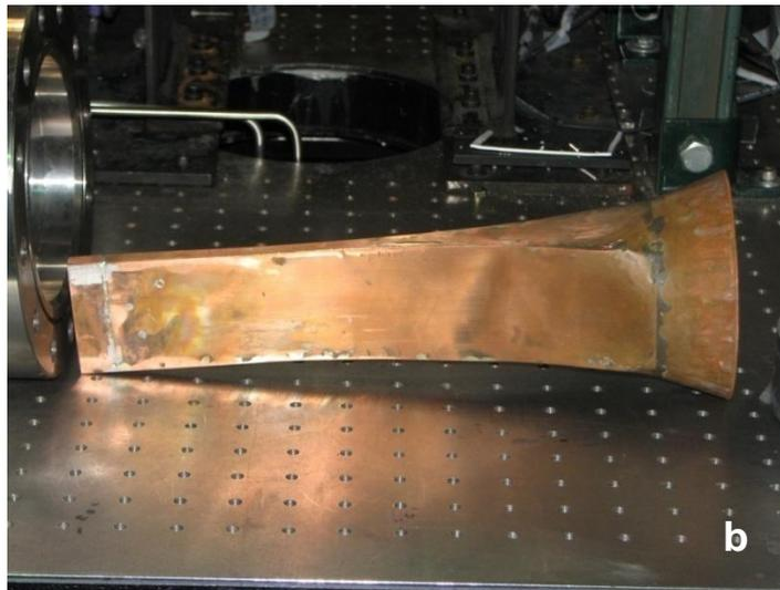
Figure 4.11. (a) One of two piezo-siren elements used to produce the acoustic field for this study. (b) Waveguide used to transmit the acoustic waves from the piezo-siren to the inner chamber.
