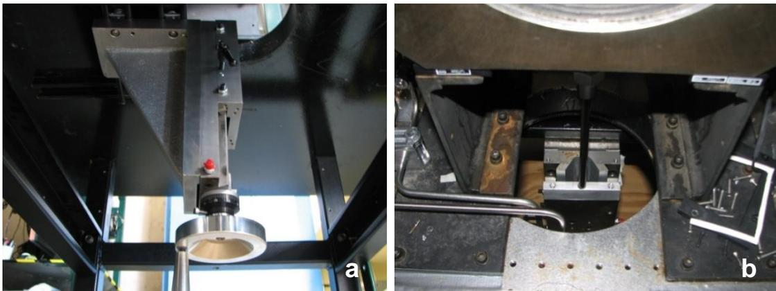
Figure 4.8. (a) Diagonal view of the mechanical stage used to move the thermocouple in the vertical direction inside the main chamber. (b) View of the mechanical stage from above. The bottom of the test chamber can be seen in the upper part of the image.
