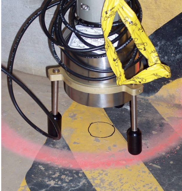
Figure 6-1. FIDLER Measurement Configuration with Dedicated Stand.
