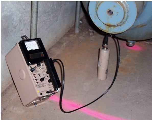
Figure 6-2. Ludlum Model 44-3 Probe (with Ludlum Model 2221 Meter) Used to Measure Area with Limited Accessibility.
