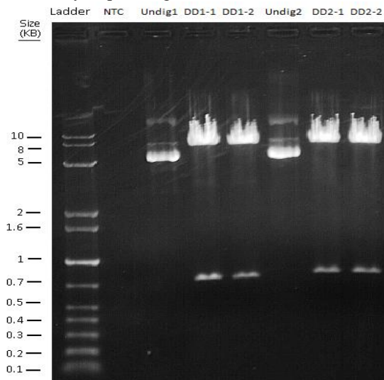
Fig. 6: 0.7% agarose gel image of pEW-bO transformants and double digestion samples. From left to right wells contain: 1Kb Plus Ladder, non-template control (NTC), undigested purified plasmid 1, replicate double-digests of plasmid 1, undigested purified plasmid 2, and replicate double-digests of plasmid 2.
