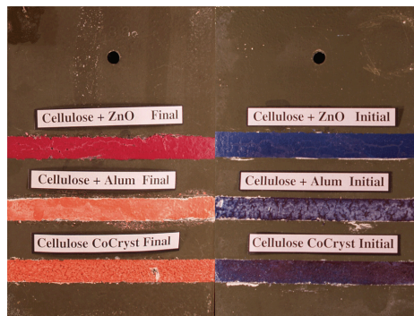
Fig. 8. Sample test panels with cellulose based formulations before and after thermal stepping.
