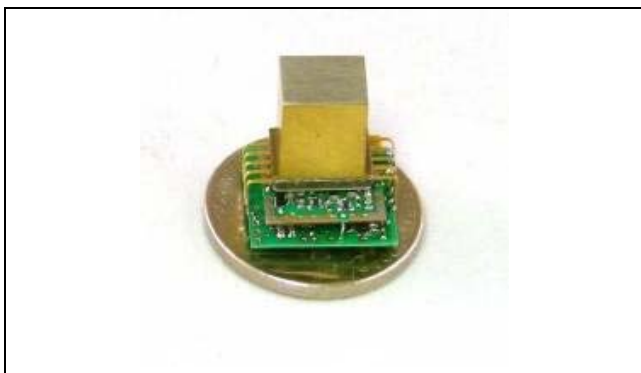
Fig.2: Compact CSAC assembly demonstrated in DARPA Phase-III CSAC Program.
