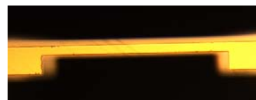
Figure 7 Optical image of the hotwire monolithically integrated on porous Si
