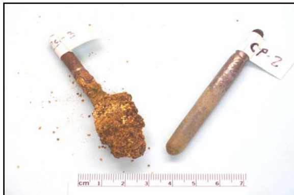
Fig. 9. Corrosion observed to uncoated (left) and coated test rods after 40-day exposure to a 3.5% NaCl solution. The dull surface of the coated rod is produced when the portland cement embedded in the glass hydrated.
