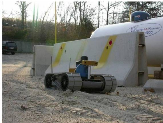
Figure 6: Wayfarer PackBot performing autonomous perimeter following
