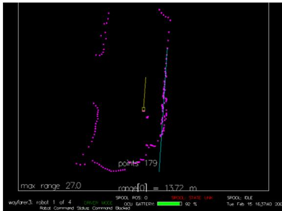
Figure 7: Hough Transform finds perimeter orientation
