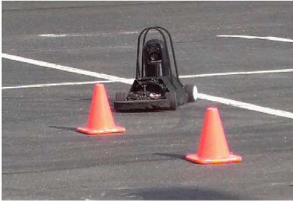
Figure 3: Surrogate UGV driving through slalom course
