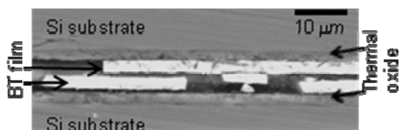
Figure 2. Cross-section SEM image of BT on Si.
