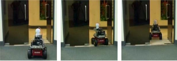
Fig. 4: Sonar perception used to avoid glass obstacles
