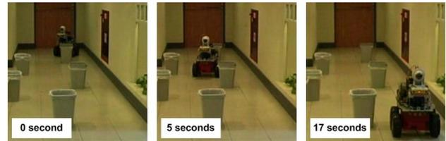
Fig. 6: Obstacle avoidance at 1m/s
