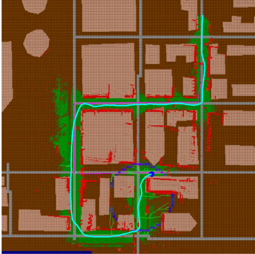
Fig 10. Path executed using route-based navigation with FCI for k=0.1 . The vehicle is able to find a route around the blockage. The trajectory is smooth and efficient, with a good compromise between global cost and local kinematic constraints.
