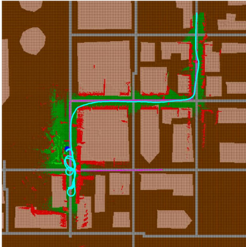
Fig 7. Path executed using route-based navigation. The vehicle is unable to find a route around the blockage using local navigation.
