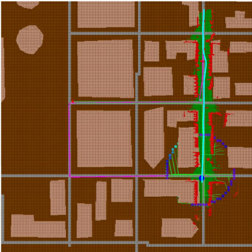
Fig 11. Path executed using route-based navigation with FCI for k=0.01 . The vehicle is unable to find a route around the blockage. Because the global costs are weighed so little, the robot ends up performing mostly locally optimal navigation, which makes the robot go almost straight and missing all turns.
