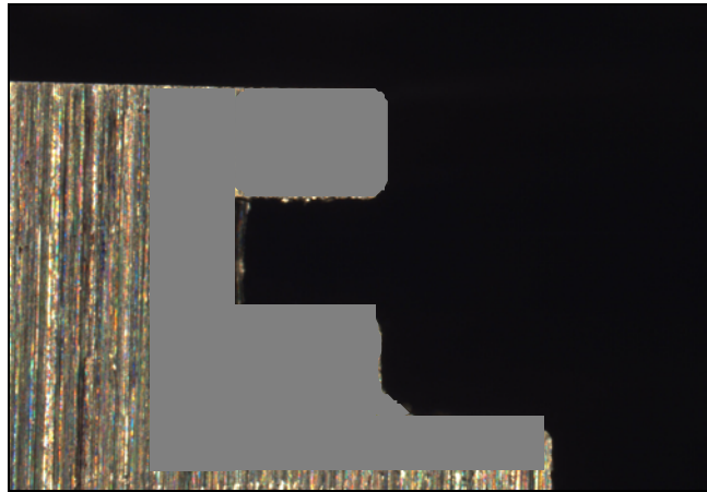
Figure 10. Cold spray material machined back to the original dimensions.
