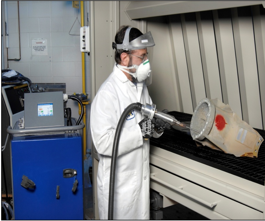
Figure 12. Operator using a Centerline Portable Cold Spray System to repair a rotorcraft component.
