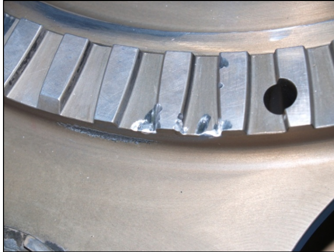
Figure 11. Mechanical damage to the splines on the Army helicopter mast support.
