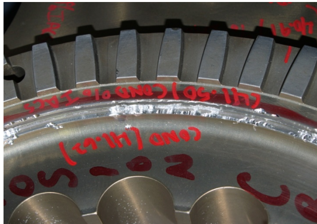
Figure 7. Mechanical damage to the snap ring groove of the Army mast support.
