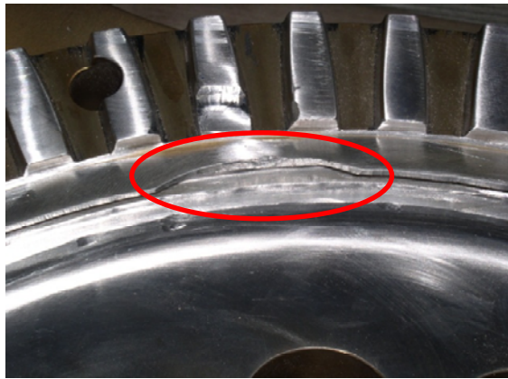
Figure 28. Mechanical damage on a snap ring groove.
