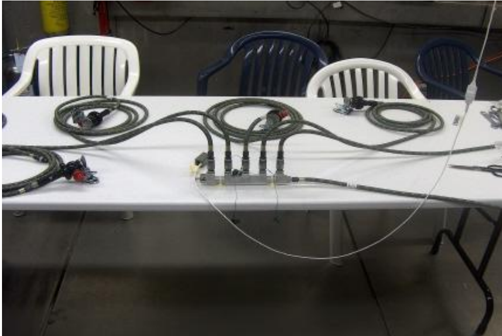
Photograph #8: POS Distribution Manifold Setup for Passenger Configuration
