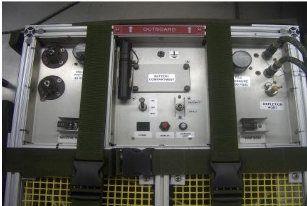
Photograph #3: Passenger Oxygen System Control Panel
