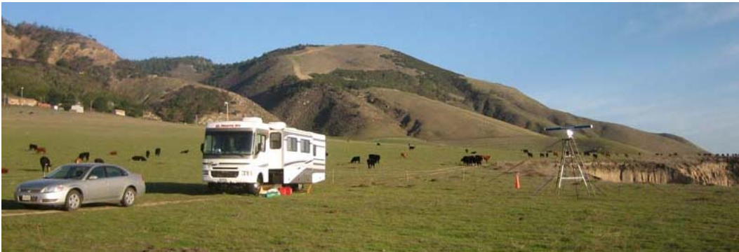
Figure 1: Furuno radar mounted on a stand near the cliff at the Diablo Canyon power plant. The RV shown at left was used to house the data acquisition and analysis computers during the experiment.
