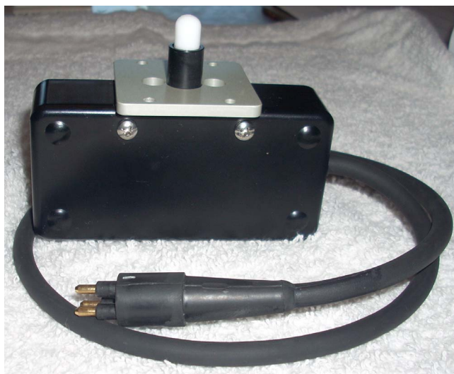
Figure 3: Monochromatic light source that provides a traceable tool to track possible sensor drift due to PMT degradation or due to the effect of biofouling. Light flux falls within the mid-range of PMT detection.
