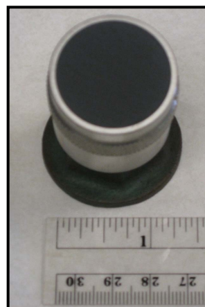
Figure 2: Three octave bandwidth broadband transducers, with center frequencies at 200 kHz, 500 kHz, and 1 MHz, that have been interfaced with the sonar boards.
