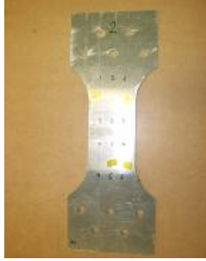
Figure 3.7: Dogbone specimen prior to sensor installation
