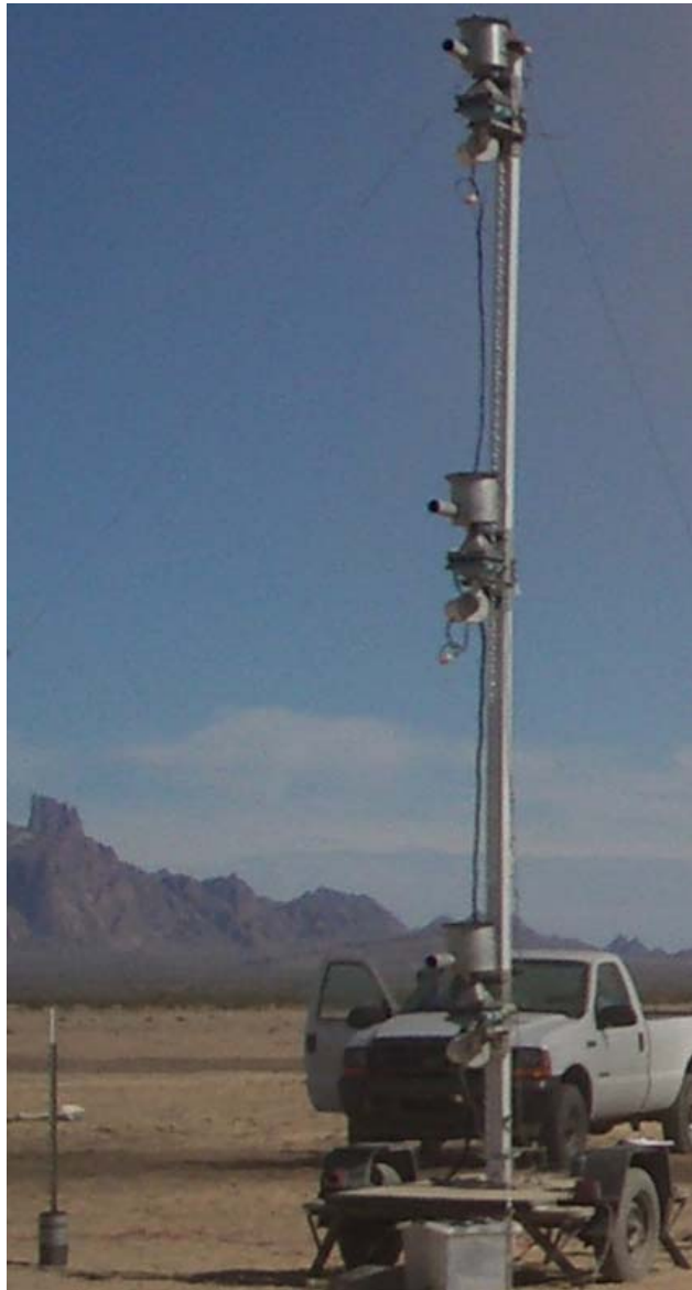
Figure 5. Dust Plume Profiling Tower (7-m Height)
