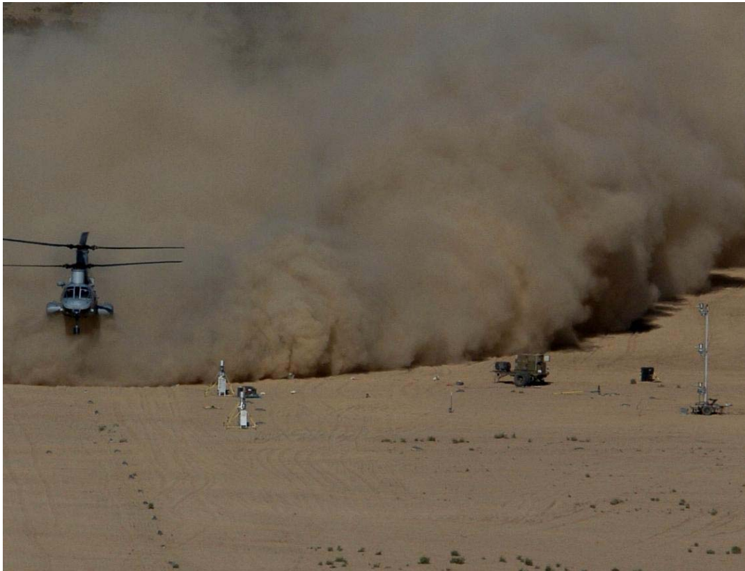
Figure 13. CH-46 Helicopter Following the Flight Path Oriented Upwind of the Samplers
