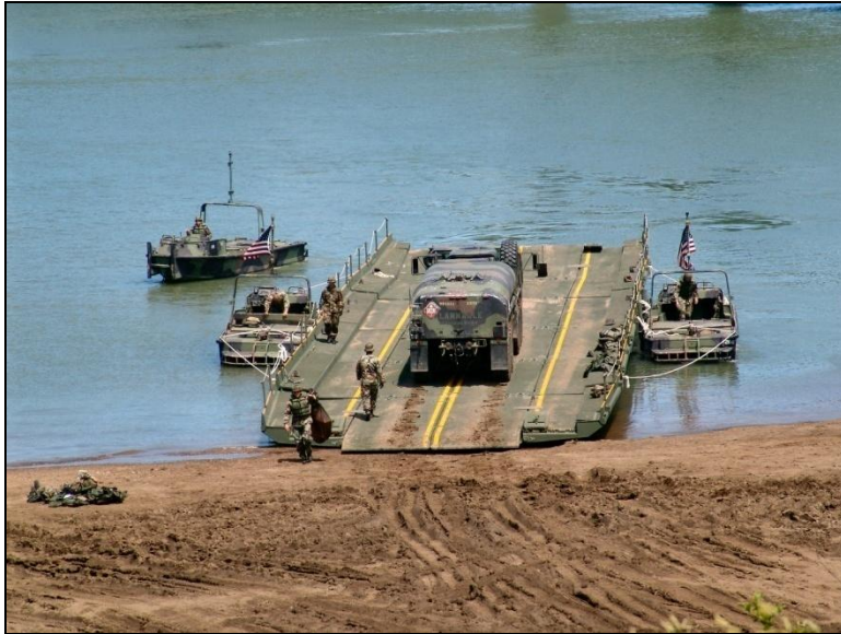
Standard Ribbon Bridge bays in Raft configuration Bridge Erection Boats provide raft propulsion
