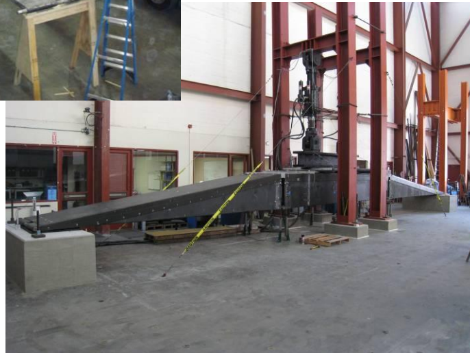
View of Complete Treadway Before ultimate failure test at UCSD
