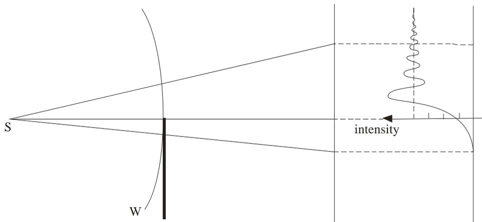
Figure 7. Diffraction Pattern at a Straight Edge.
