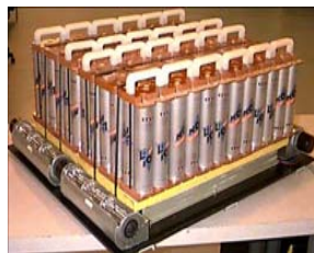
Battery Pack w/ Integrated Heat Exchanger
