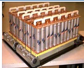
Battery Pack w/ Integrated Heat Exchanger
