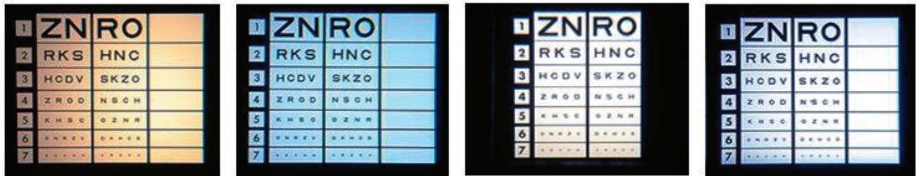
Figure 9: Photos of target slides taken through the optics of each device with a Nikon E8700 digital camera. From left to right: Optec 2000, Optec 5000, Titmus 2A, and Titmus i400. (Note: These images are to demonstrate color differential, not to accurately depict the subject's view of the test slides.)
