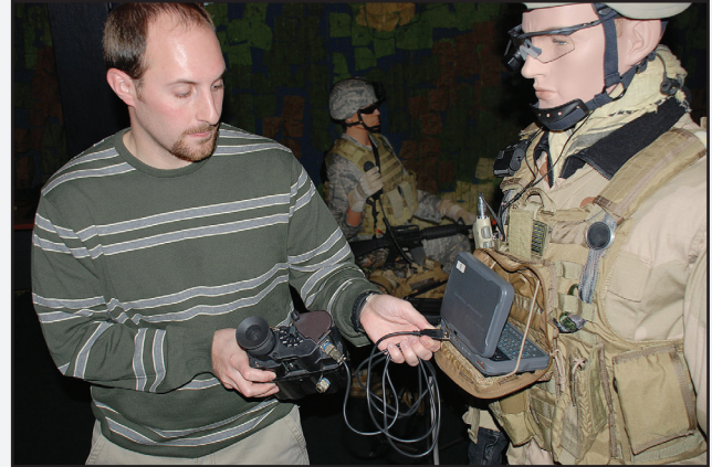
AFRL project engineer Greg Burnett (left) demonstrates the user-friendly Grabs-M cable, the design of which enables combat controllers to quickly and efficiently transfer digital coordinates from a laser range finder to a computer in the field (photo by AFRL's Chris Gulliford).
