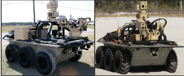
The Defender, a robotic platform that performs reconnaissance, surveillance, targeting, and threat neutralization tasks in support of base defense operations
