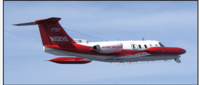
Calspan Learjet equipped with the EO cameras, AI-130 radar, and airspace deconfliction technologies that make up the SAA system test platform (photo courtesy of Calspan Flight Research)
