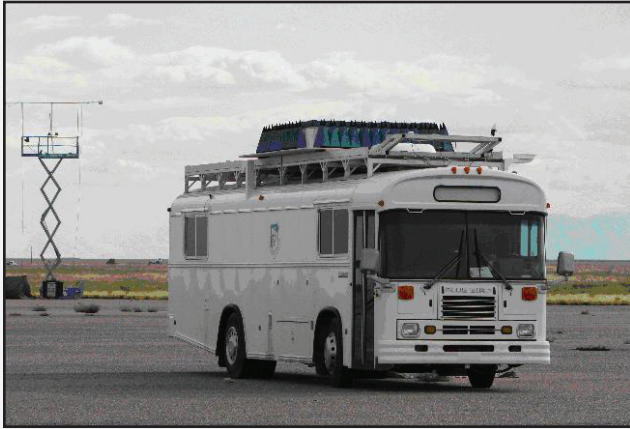
Next-generation GPS/INS antijam technology mounted atop an AFRL mobile test vehicle to demonstrate weapons navigation capabilities
