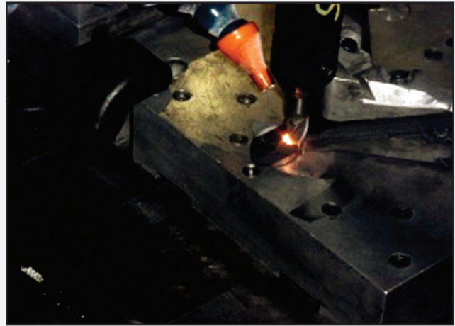
Accelerated machining of CMCs
