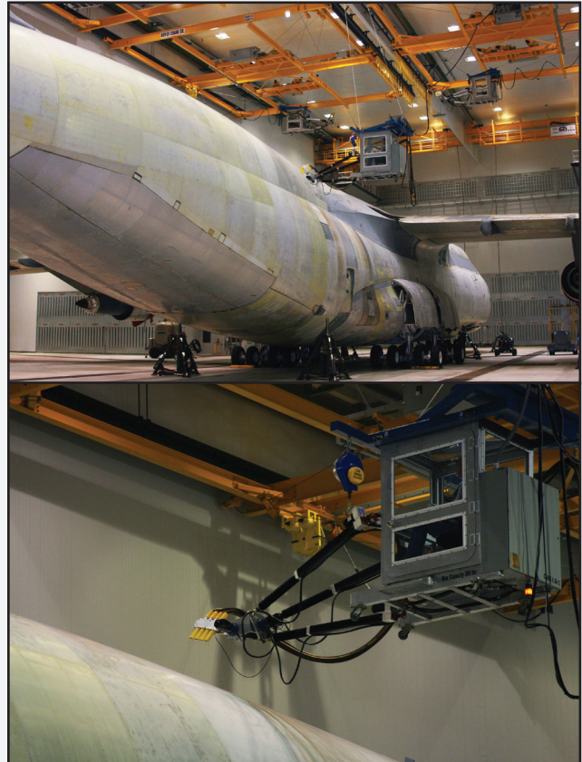
RoboCrane/AMP in use for aircraft coatings removal
