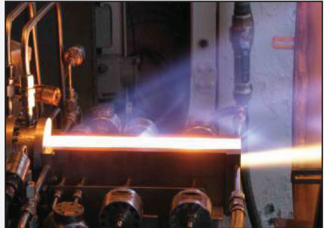
A cooled CMC panel undergoes a hot-fire test at the National Aeronautics and Space Administration's Glenn Research Center.
