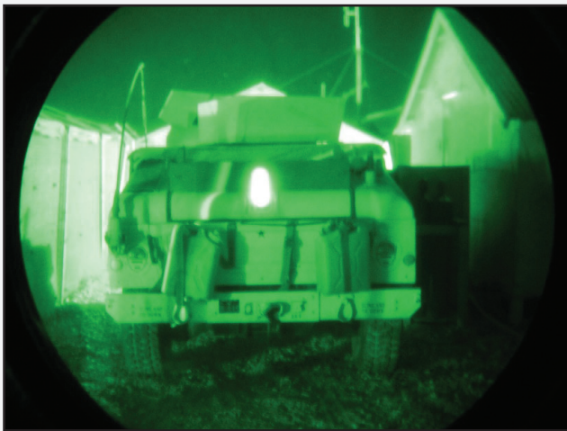
Military vehicle marked with TRON I (glowing strip in the center) and TRON III, as viewed through night vision goggles
