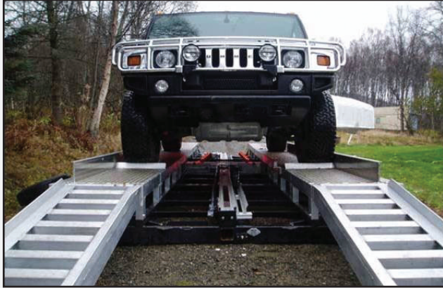
A sport utility vehicle parks on ramps that permit MUVIS to photograph its undercarriage.
