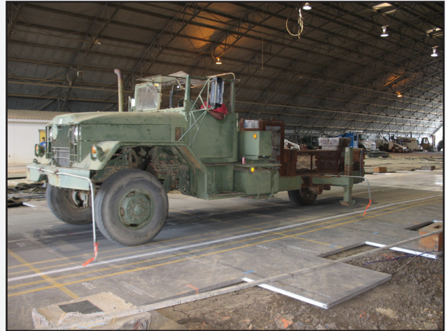
Tests of weight-bearing capacity being conducted using a load cart
