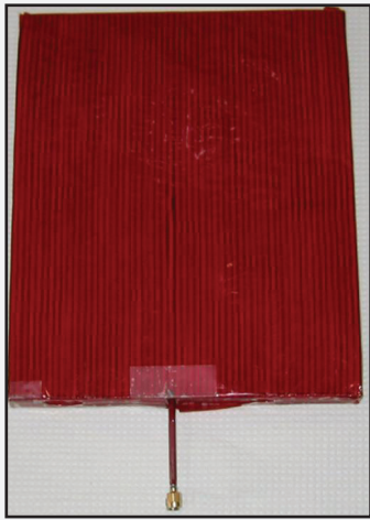
Dipole antenna inserted into AFRL's near-zero [refractive] index material
