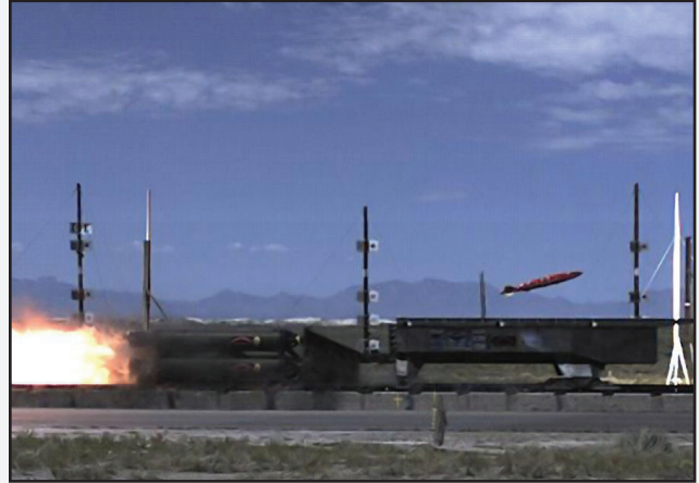
Researchers at the Holloman High-Speed Test Track (Holloman Air Force Base, New Mexico) succeed in accomplishing the first-ever test release of an MK-82 JDAM on a rocket sled traveling at supersonic speed—Mach 2 (image courtesy of Air Force and Boeing).
