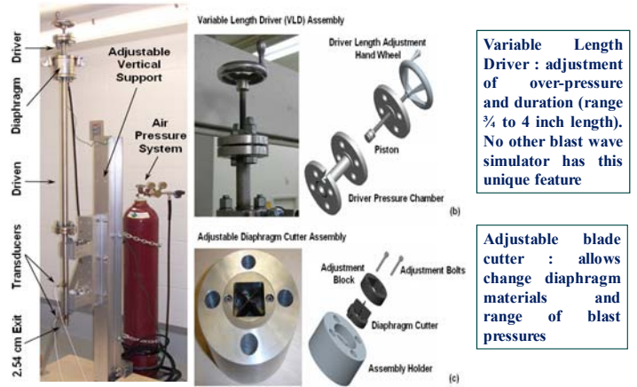
Fig.1B Blast Generator Set-Up.
