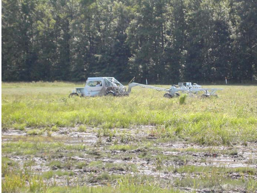
Figure 1. Demonstrator system, magnetometer (MAG) MTADS/towed.
