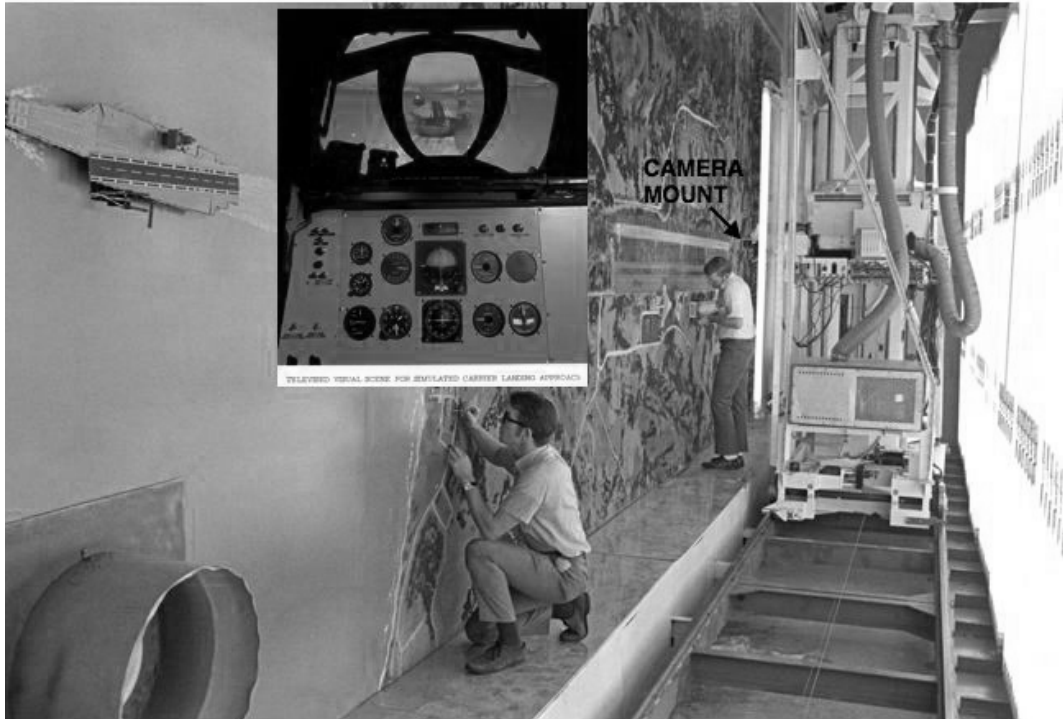
Figure 2. NASA Ames' Visual Flight Attachment system (c. 1971). A video camera (initially black-and-white, later color) was mounted at the rail-based tracking system shown on the right. The camera was "flown" over the terrain model board via instructions from the simulator cab. The inset shows an example of the imagery displayed to the pilot, in this case for a landing approach to the aircraft carrier.
