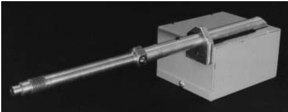
Figure 2. A fiber optic probe, referred to as the CAMES probe, was used at NAVSEAIHMD to detect concentration of tracer in RTD and other processing experiments
