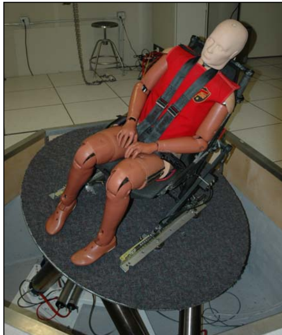
Figure 1. The Multi Axis Ride Simulator
