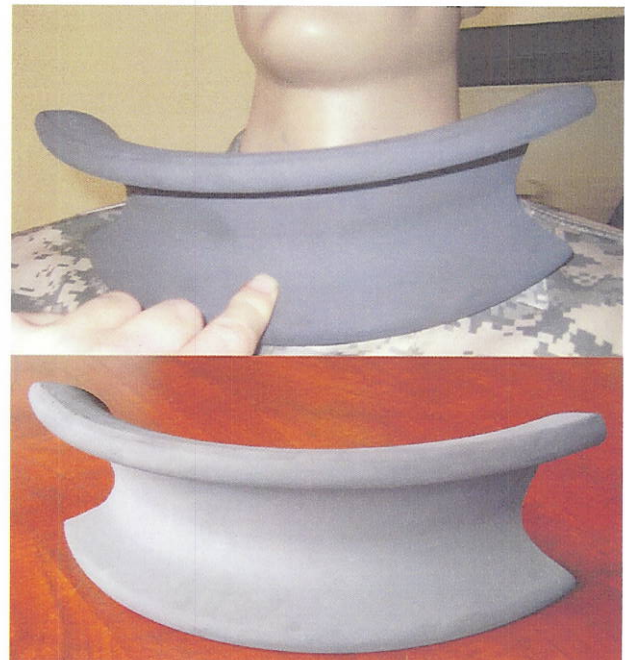
Figure 5. Complex shaped part of B 4 C manufactured by Verco Material via pressureless sintering using conventional powders.
