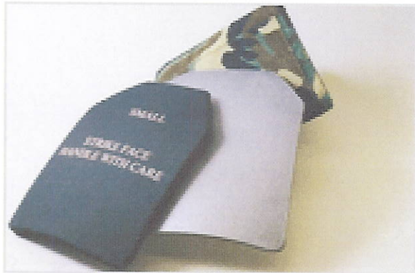
Figure 4. B 4 C plates formed via hot pressing with a curved shape.
