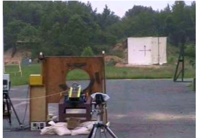
Figure 12 Range test setup of guided grenade at ARL.
