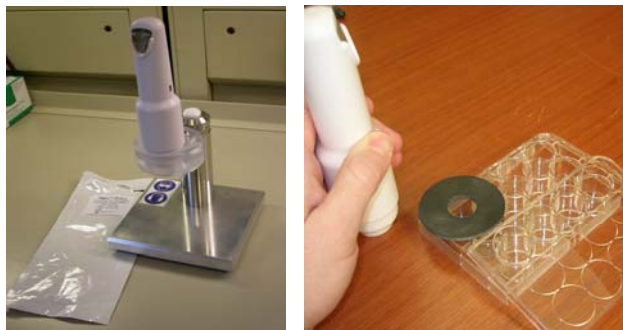
Fig. 4. Recovery and detection of the DNA vaccines contained in the PMED devices. The HTNV and PUUV DNA vaccines were manufactured in single use hand-held disposable PMED devices and packaged in sealed pouches containing a desiccant (A). For potency and stability tests, a PMED device was discharged into one well of a 12-well plastic plate containing either ethanol (for the quantitative assay) or into mammalian cells (for the qualitative assay). To ensure complete delivery, a neoprene washer was placed over the well before activation of the device (B). DNA was recovered and expression assessed.
