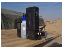
Figure 8 An M-25 Beta DMFC system evaluated in Iraq
