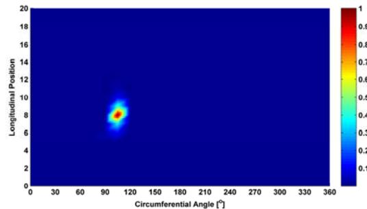
Figure 2. Normalized similarity values over the surface of the casing for an impact at a longitudinal position of 8 and a circumferential angle of 105°.
