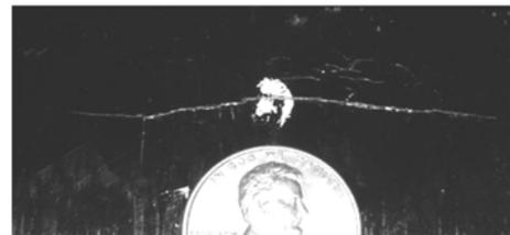
Figure 5. The damage produced by the impact reproduced in Figure 4.
