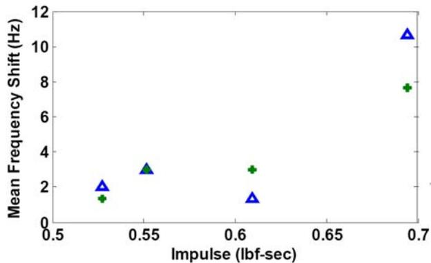
Figure 7. The mean frequency shift of the third natural frequency according to the reproduced FRFs (+) and the FRFs found via modal impact testing ( $\Delta$ ) plotted against the impulse of the applied force.
