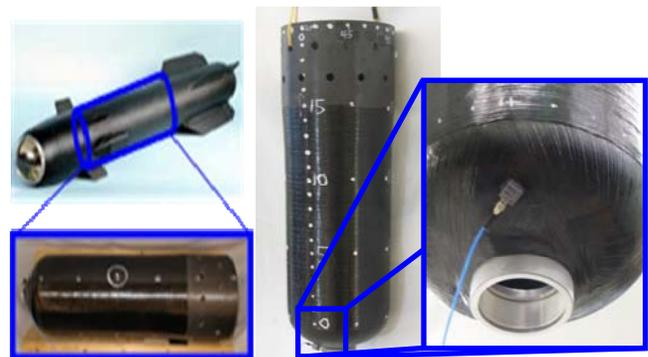
Figure 1. Carbon filament wound missile casing with the attached triaxial accelerometer.
