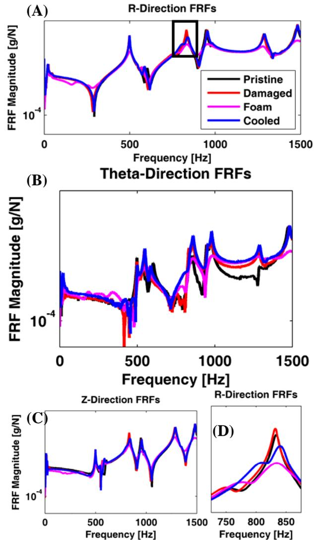
Figure 9. Experimental frequency response functions acquired using modal impact testing in (a,b,c) multiple directions with close up in (d) of peak in (a).
