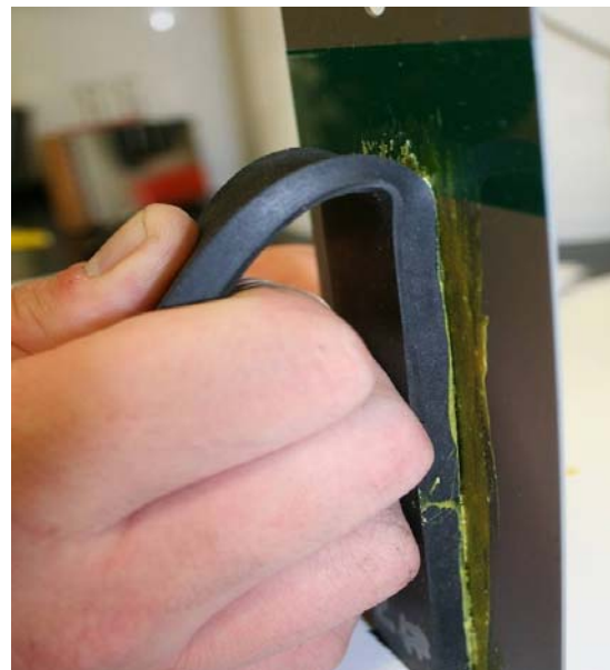
Figure 10: Photograph showing that no adhesive failure occurred baseline 3M-1357L.
