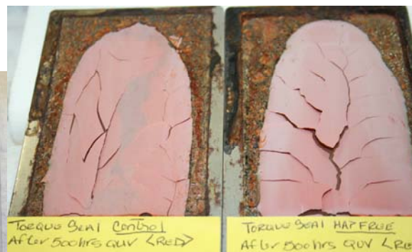
Figure 5: Torque Seal QUV results after 500 hrs exposure.
