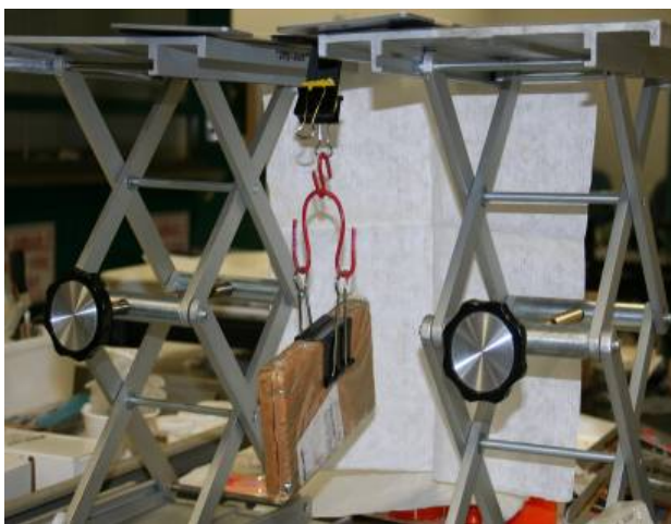
Figure 9: Basic strip adhesion set-up for MMM-A-121.
