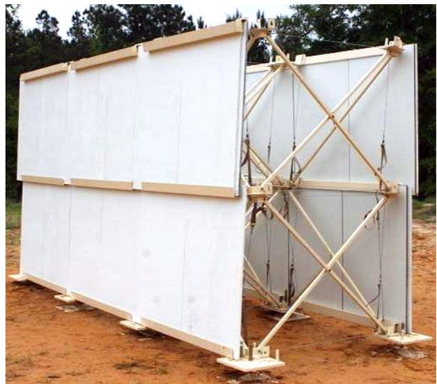
Figure 3 Completed MPS section with armor panels
