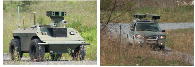
Figure 2. Our UGVs with LADAR sensors
